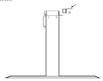
> The side plates (5) were fixed on the column with M6 countersunk screws (holding)
