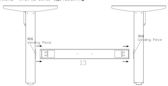
➤ Note: the two table frames should be placed with welding blocks facing inward, otherwise the connecting rod to the table cannot be installed
