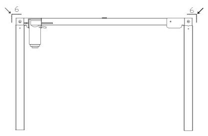
➤ Will Hexagonal drive assembly (7) the two locks on the section slightly loosen that can pull out the inside of the hexagonal rods, again stab motor side short hex-drive components in the hexagonal rods (left), then after the completion of hexagonal transmission components in long hexagonal rods out of stab without motor column (right), the final adjustment of aluminum tube to appropriate position lock two day after locking
