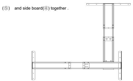
> Third, As shown in the figure below, place the column(①) in the frame(③),adjust the frame to the proper distance,fasten it with screws(⑫and③)
