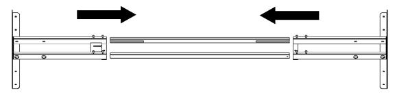
The third, stretch the cross frame to the right length ,place the cross frame on top of the panel. Lock panel and frame with Flat head screws (Item12).
